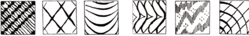
– Generation of sound patterns of classical music on the screen of a Nipkow television system (1930) by Fritz Wilhelm Winckel. Source: Fritz Wilhelm Winckel, "Vergleichende Analyse der Ton-Bild-Modulation," in Fernsehen , no. 4 (Berlin 1930), 171–175, here 173.
